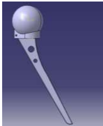
Fig. 2: CAD modeling of Hip Joint using CATIA
